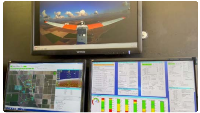
Flight tracking, Command and Control (C2), and telemetry data over L-band satellite communications. The top monitor displays the tail camera streaming over LTE.
